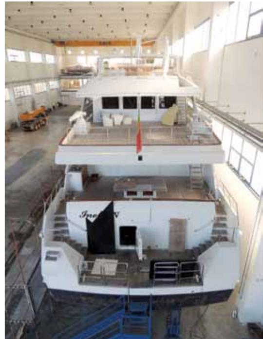
ABOVE: *Ineke IV* suffered from noise and vibration issues. BOTTOM: Lengthening the yacht's stern and upper deck created a more pleasing aesthetic overall.
